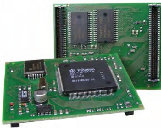
The ISM-167 offers a capable 16 Bit microcontroller of type SAB-C167CR together with a Flash- und RAM-storage enlargement, a serial FRAM and a real time clock in a compact and consistent format of our ISM-family.
