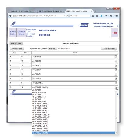
Configuration page for a modular chassis which allows a choice of virtual PXI modules
