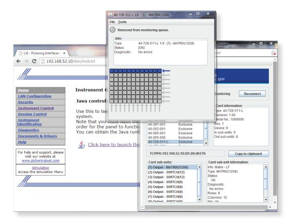
The 60-901 selected chassis provides soft front panels to enable manual operation through the web interface, in this example for a 40-726 matrix module.
