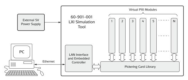
Simulation of Pickering Interfaces PXI modules using the 60-901 LXI Simulation Tool provides an application development platform. A simple Ethernet lead is the only physical control connection required.
