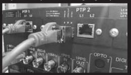
This is back view of Time Server with 1-4 Expander cards. Cards are autonomous GRANDMASTERS. Only card #1 can be set to operate SLAVE mode, but all 4 can act MASTER. Cards support PTP profiles: DEFAULT, ENERGY, TELECOM. The National Physical Laboratory in London (UK) confirms 50ns accuracy of synchronization to cesium clock UTC-NPL.
