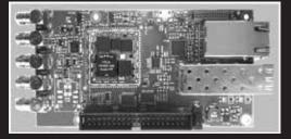
On the right side are output pares of L AN3-4, 5-6, 7-8, 9-10. On the left side there are internal analogue sync interfaces. They are internally connect via analogue signals SyncBUS.
