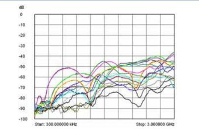
**Isolation Plot** - This is a measurement of the amount of signal that is transferred from the input to the output of a switch with that particular path disabled or in the "off" condition
