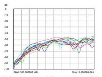
Crosstalk Plot Between Ports - In this case signals are applied to the input of a switch path with a terminated output. The signals picked up by the unused channels within the same switch bank are measured.
