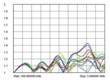
**VSWR Plot** - This is created by terminating the output of the switch with the characteristic impedance and inserting a range of frequencies into the input. The amount of signal reflected back to the input is calculated as a ratio. In a perfect system, all the input power would be transferred into the termination giving a VSWR of 1:1. Typically a switch is usable with a VSWR of up to 1.5:1 for a given frequency.
