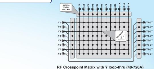
Crosspoint Matrices use SPST relays at each connection point to form X to Y signal paths. PCB layouts are carefully optimized for the best RF perfomance and isolation relays are included in
