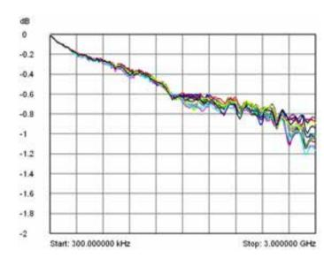
**Insertion Loss Plot** - This is a measurement of how much power is lost through a switch. A range of frequencies is inserted at the input and the level at the output is measured and plotted as dB below the input. In an ideal system this would be zero, but in practice consistency between paths is important. Careful RF design practices ensure that each switch path of a module has a similar amount of loss.
