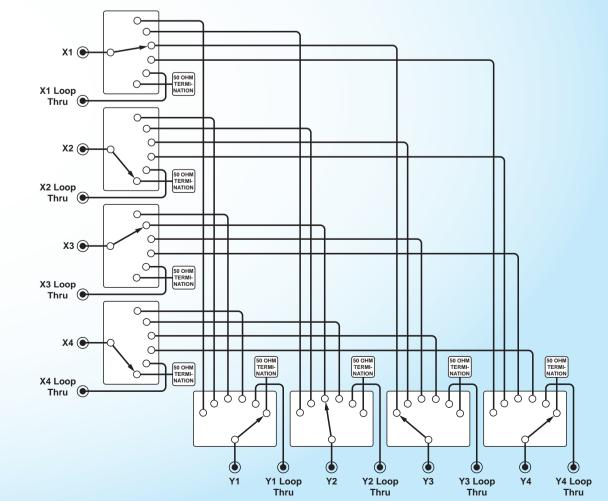
4x4 Microwave Matrix with termination & loop-thru constructed using 6 to 1 multiplexers (60-750)
