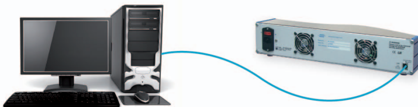
Fig. 2.1 - PC and LXI Device with direct Ethernet connection
