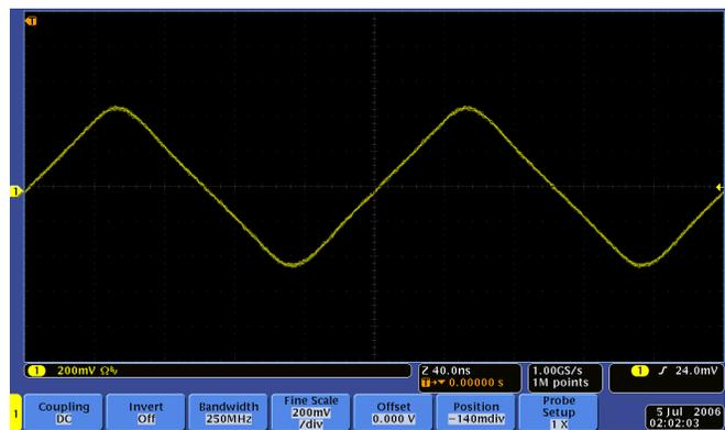
Triangular Waveform at Frequency of 5MHz
