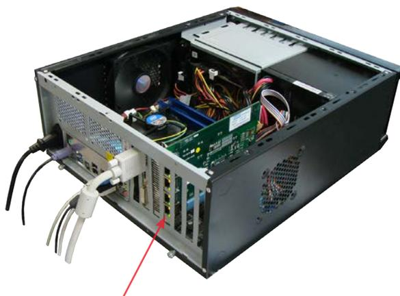
**A standard PC with Pickering PCI card fitted to the Motherboard. Outputs unconnected.**
