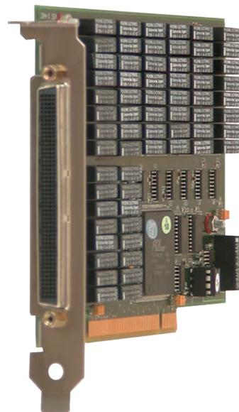
The 50-110/115 range of switching cards are available in both Changeover (SPDT) and Normally Open (SPST & DPST) configurations. Connections are made via a front panel 200 pin female connector.
