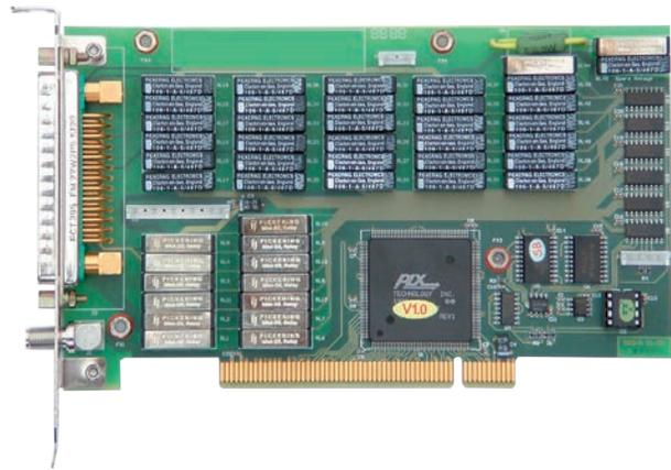
The 50-350 is a Short PCI Card designed as a high voltage multiplexer for use in a Submarine Cable Testing Application.
