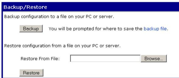
The configuration of this digi device can be saved to a file. This configuration file can be used to configure this or any other digi device module.
