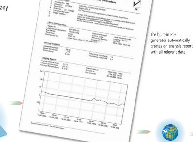
The analysis report in the form of a PDF file can either be saved locally or on a companyown network, printed or sent by email. All raw data is tamper-proof embedded in the PDF file. (Detailed analysis with elproLOG software possible)
