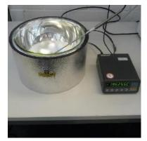
Check LN2 temperature with the reference instrument. Depending on the atmospheric pressure, it will show a temperature between -195 °C and -197 °C. Cover the top with a styrofoam to prevent from strong boiling.
