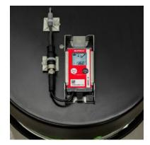
After 10 minutes, check temperature of LIBERO CE. For a new system, the reading should be within +/-2° of the reference instrument, i.e. between -194° and -198°C. Acceptable tolerance may be higher depending on the quality of the used Pt100 probe.
