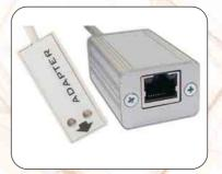
LAN adapter for communication with the PC via LAN network
