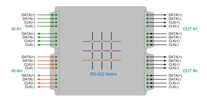
The KSD0511 is capable of switching data rates up to at least 10 Mbps.
