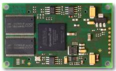
Furthermore the ECUcore-EP3C comes equipped with 2 MiB SRAM, 1 MiB Serial Flash for application storage and
