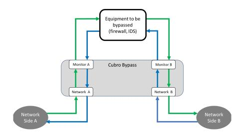
Traffic Flow in failure mode (electrical power and/or configurable triggers)
