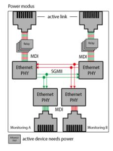
Power autage modus UIIIII active link MDI Ethernet Ethernet SGMI PHY PHY Ethernet Ethernet PHY PHY MDI Monitoring A Monitoring B active device needs power
