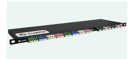
The Cubro OPTOSLIM TAP Series offers real-time monitoring access to a physical optical data link with zero performance degradation or disruption. Since an optical TAP is fully passive (no power supply needed) there is no risk associated with placing them inline on an active link. The TAPs do introduce additional optical power loss on the active link which varies with the split ratio used; otherwise, the TAP is completely transparent to the network.
