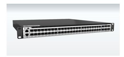
The Packetmaster EX48400 is a high performance network packet broker that aggregates, filters, duplicates, load balances network traffic to security, monitoring and management tools based on 4500 possible rules. The Packetmaster EX48400 supports OSI Layer 2, Layer 3 and Layer 4 header modifications including stripping, adding, and modifying VLAN tags, MPLS labels, MAC addresses, IP addresses and Port numbers.
