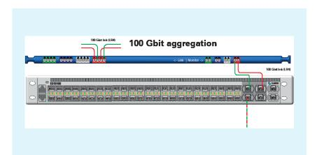
The EX48400 receives traffic from a 100G live link via the monitor ports of an inline TAP.
