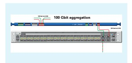
The EXA32100 receives traffic from a 100G live link via the monitor ports of an inline TAP.
