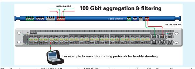
The Sessionmaster EXA32100 supports 4000 filters that can classify traffic. These filters can be used to redirect a selected part of the traffic to a low bandwidth monitoring tool, such as a 10G packet analyzer to troubleshoot an issue on a 100 Gbit link (such as a routing problem).
