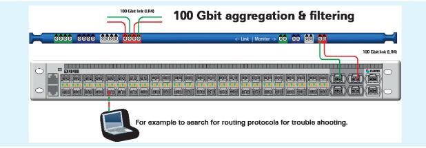
The Sessionmaster EXA48600 supports 4000 filters that can classify traffic. These filters can be used to redirect a selected part of the traffic to a low bandwidth monitoring tool, like a PC with Wireshark to trouble shoot an issue on a 100 Gbit link (such as a routing problem).
