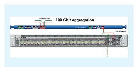
The EXA48600 receives traffic from a 100G live link via the monitor ports of an inline TAP.
