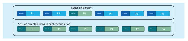
**Raw packet tagging:** Tagging the identification information in the "MAC" field of raw packet header. FlowVista supports tagging buffering feature. For example: packet A is in front of packet B in the same session and packet B carries the signature. When FlowVista identifies the signature carried by packet B, it can still tag packet A with the signature information.
