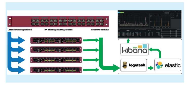
The Cubro FlowVista probe can be also used to generate metadata from the network and feed a big data application. As one example of such an installationthe picture shows 3 open source applications (ELK ore kibana stack) which can be used to build a powerful and flexible collector.
