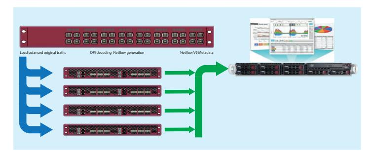
This drawing shows a typical solution to monitor a huge amount of traffic, in this case more than 250 Gpbs. The traffic is received via TAPs to the EX32100 from various interfaces. The EX32100 is aggregating, filtering and load balancing the traffic to 4 FlowVista Probes, each handling 60 - 70 Gbps traffic.
