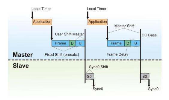
The local application is started with a local timer. The local timer is shifted to the DC base Time by the sum of the following times:
